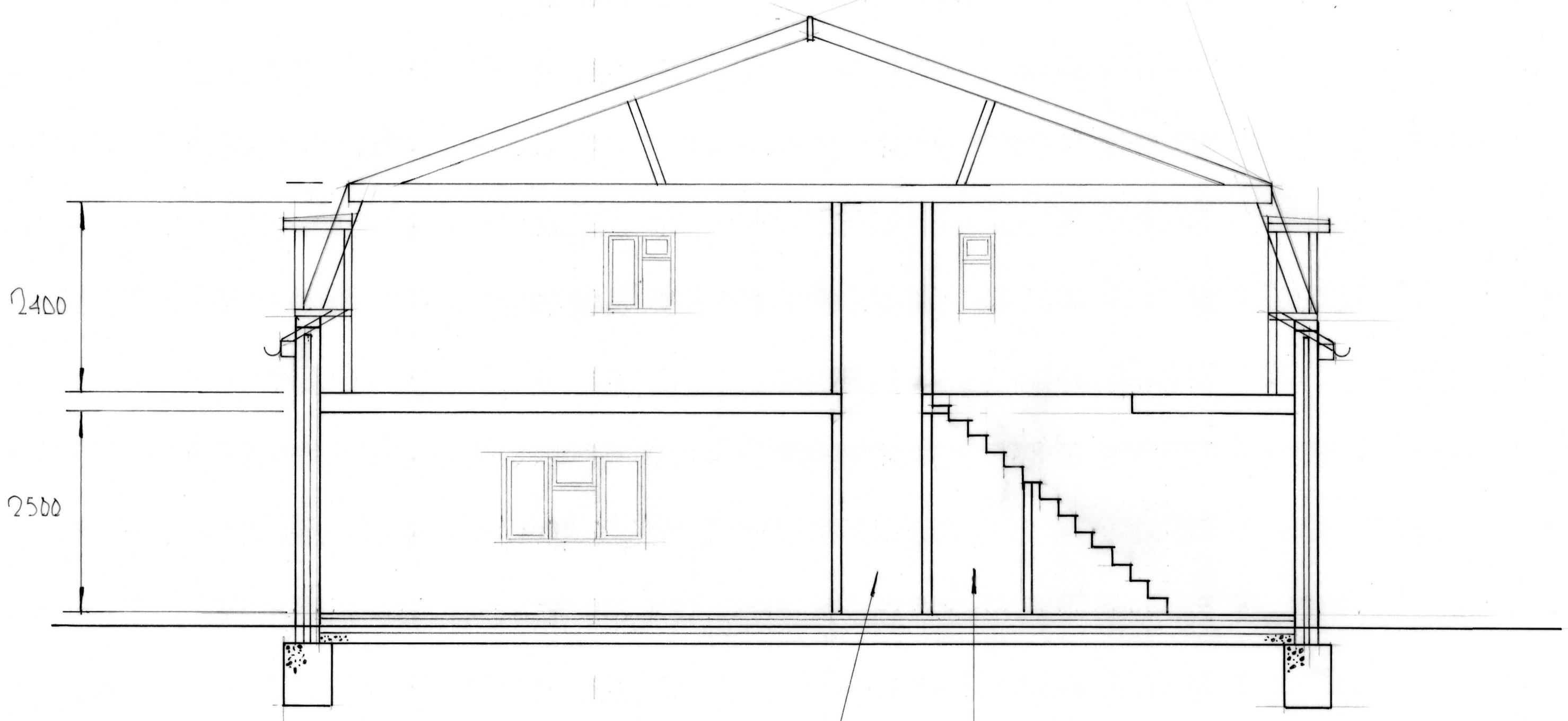
This area is set aside for a Mobility Lift from Ground to First Floor. Exact Dimensions for the lift and Landing Area will Be Submitted at a Later Date.
