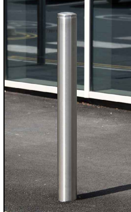
Entrance Bollards Location: Externally to office area Range: Marshalls RS001 (or similar approved) Finish: Stainless steel Note: Bollards to be fixed in place to substrate beneath finished surface, with block paving cut to suit to conceal fixings.
