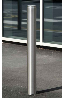
Entrance Bollards Location: Externally to office area Range: Marshalls RS001 (or similar approved) Stainless steel Bollards to be fixed in place to substrate beneath finished surface, with block paving cut to suit to conceal fixings.
