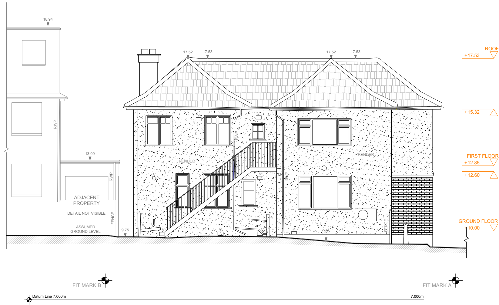
EXISTING REAR ELEVATION
