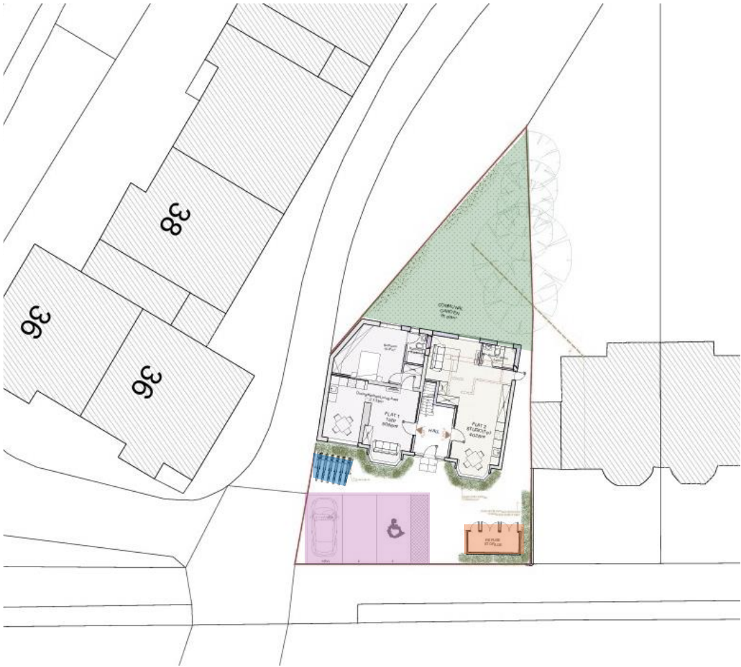
FIG 10. GROUND FLOOR PLAN HIGHLIGHTING GARDEN SPACE, CAR PARKING, CYCLE STORE AND REFUSE STORAGE
