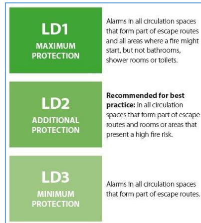
Figure 1 Fire alarm coverage for dwellings
