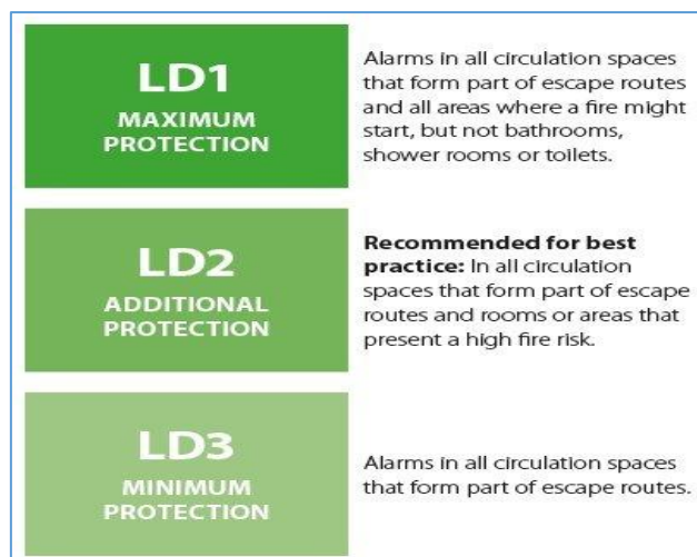
Figure 1 Fire alarm coverage for dwellings
