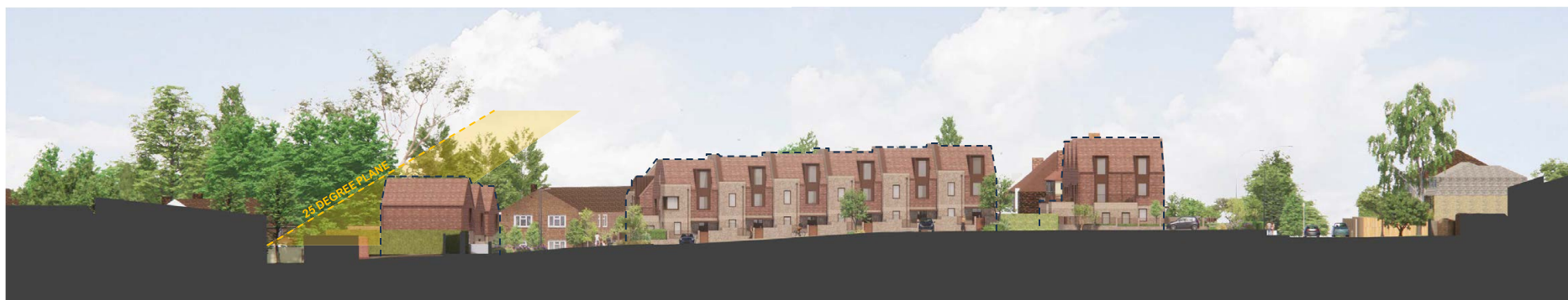
Proposed Haydon Drive North Elevation – designing for daylight using appropriate separation distances, orientation and roof pitch
