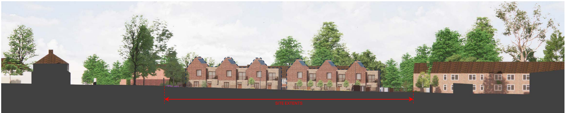
Proposed Haydon Drive West Elevation – 2-storey terraced houses with gable roof form
