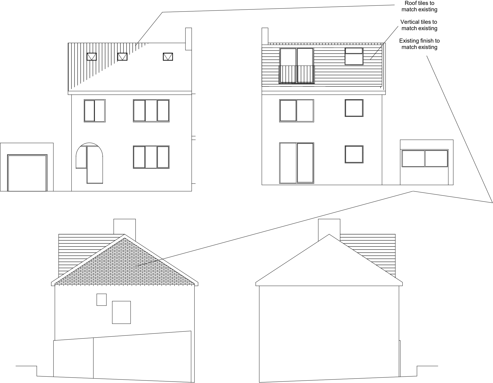
PROPOSED FRONT / REAR & SIDE ELEVATIONS Scale 1:100
