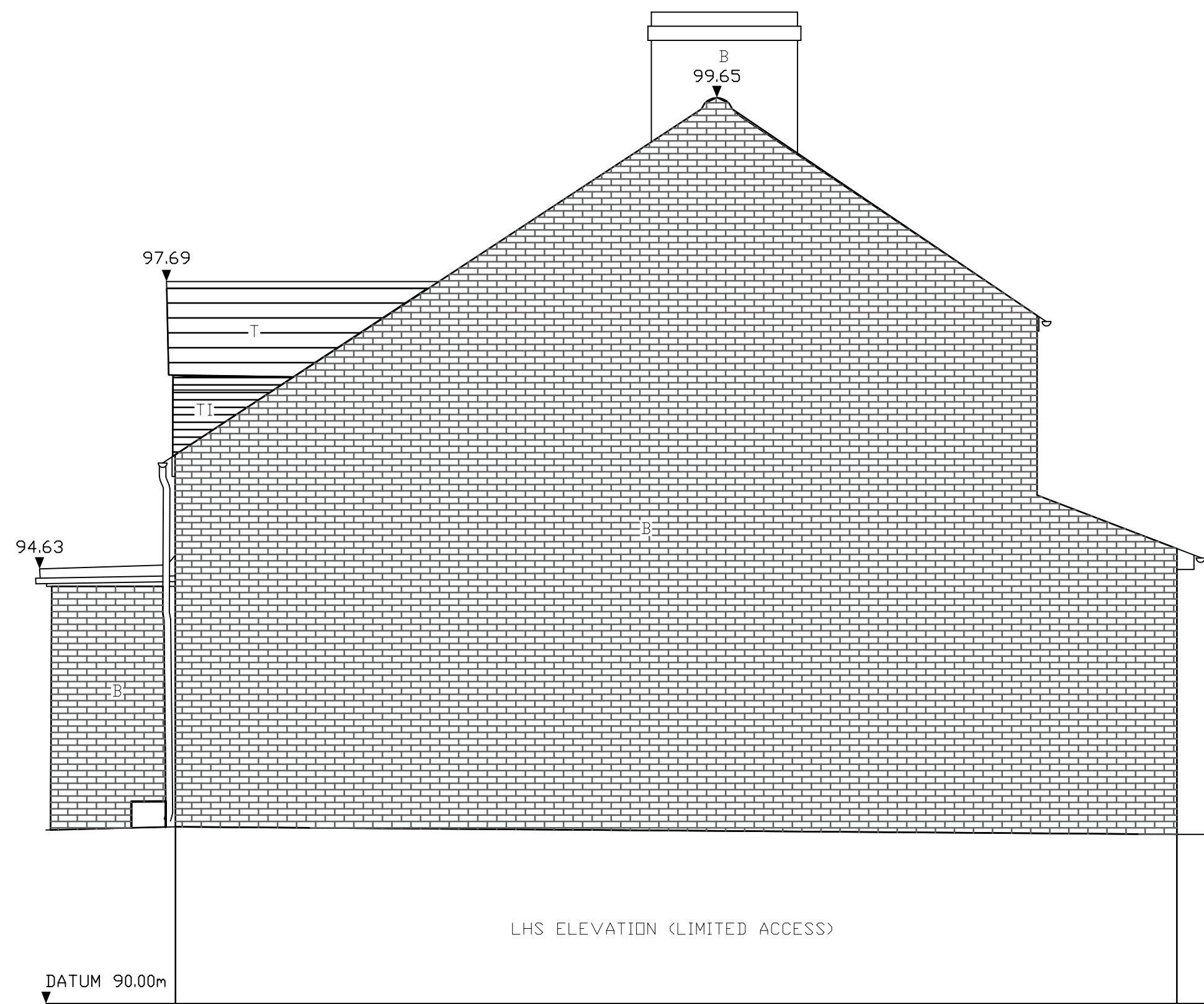
06 PRE EXISTING SIDE (EAST) ELEVATIONS
