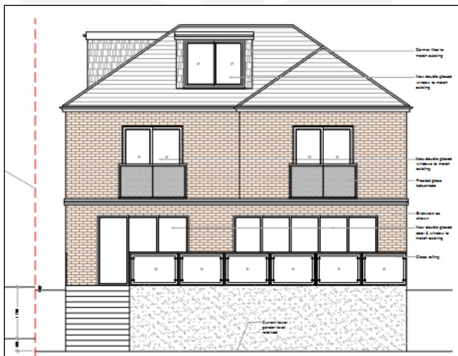
Fig. 4: Proposed Rear Elevation - DE Architectural Consult. Ltd
