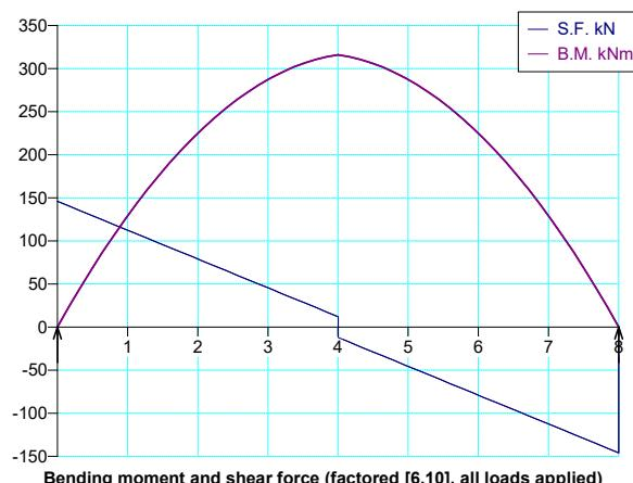
Beam calculation to BS EN1993.1.1 using S355 steel
