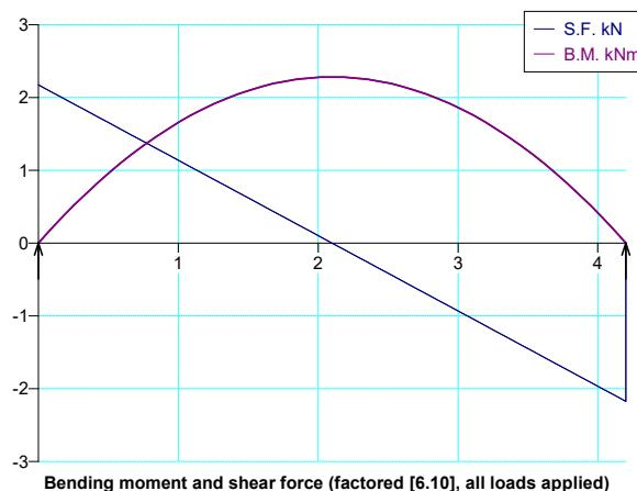
Timber beam calculation to BS EN1995-1-1 using C24 timber
