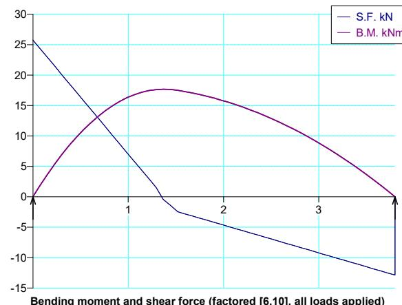
Beam calculation to BS EN1993.1.1 using S355 steel
