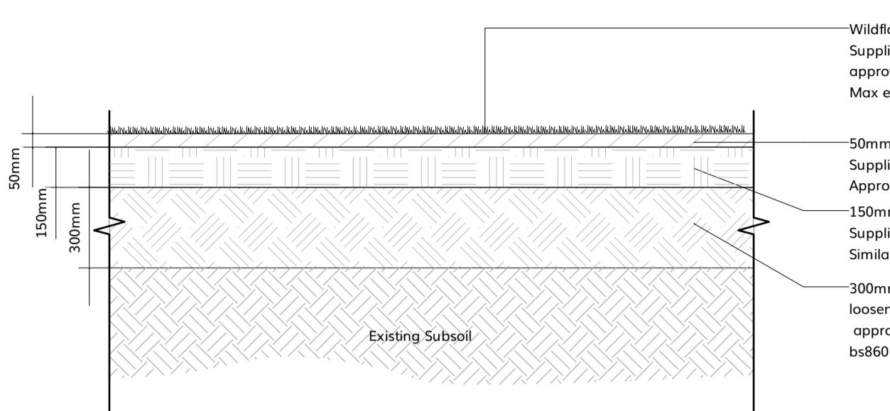
D13 Typical Detail - Typical meadow build up - Section
