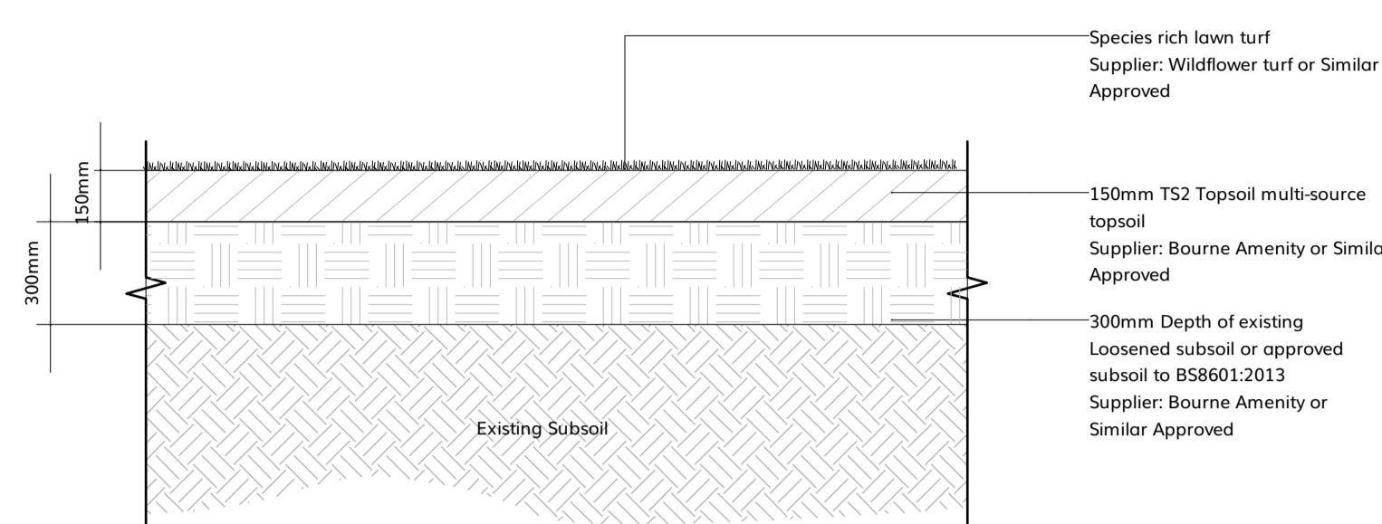
D12 Typical Detail - Typical lawn build up - Section
