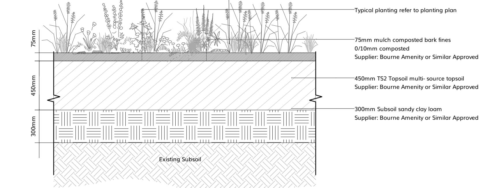
D14 Typical Detail - Planting build up - Section
