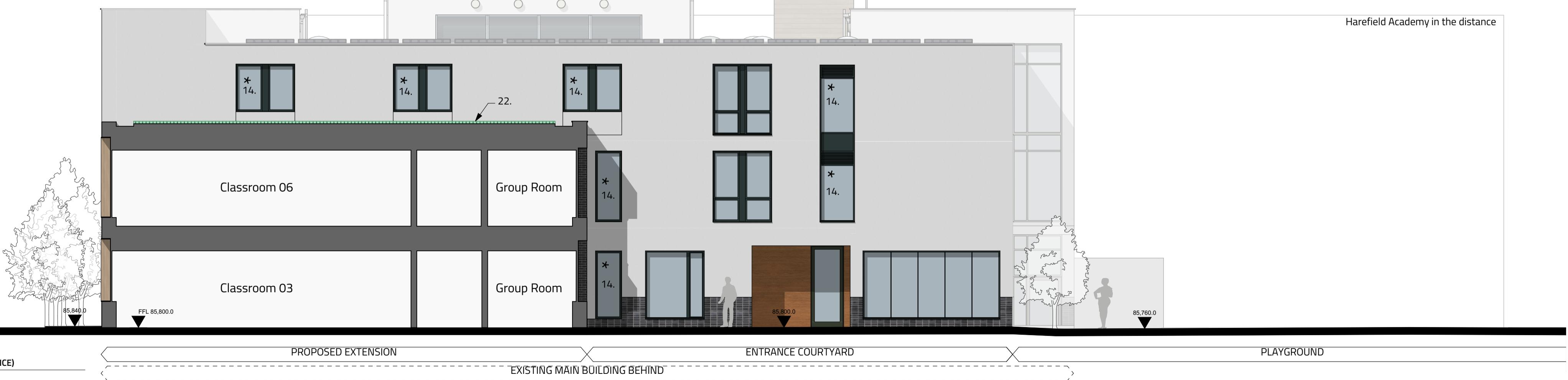
\* Existing windows identified with an asterisk are to be altered or replaced. Where shown, windows to be fitted with acoustic ventilation louvres to provide improved teaching spaces. Finishes to match existing.
