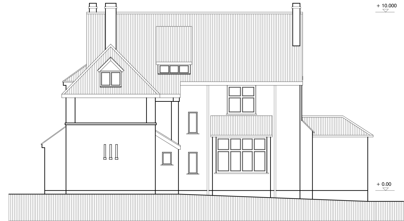
SOUTH ELEVATION AS EXISTING (NO ALTERATION)
