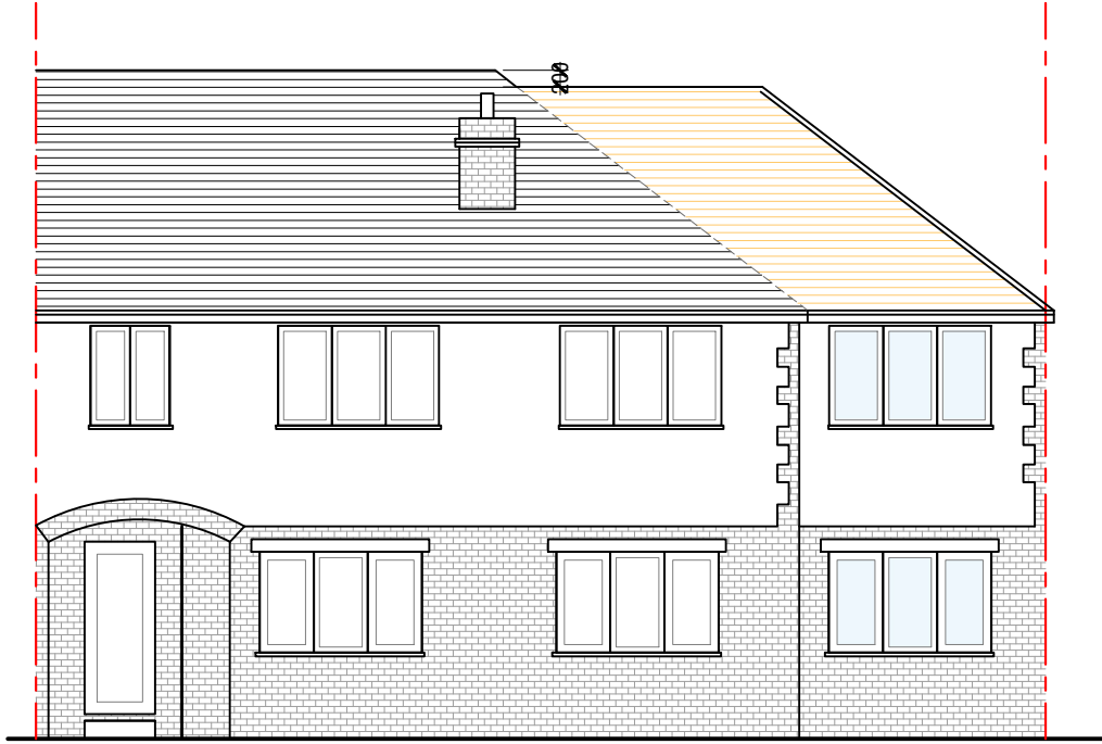
PROPOSED FRONT ELEVATION Scale 1:100
