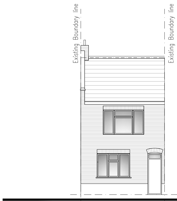
EXISTING FRONT ELEVATION
