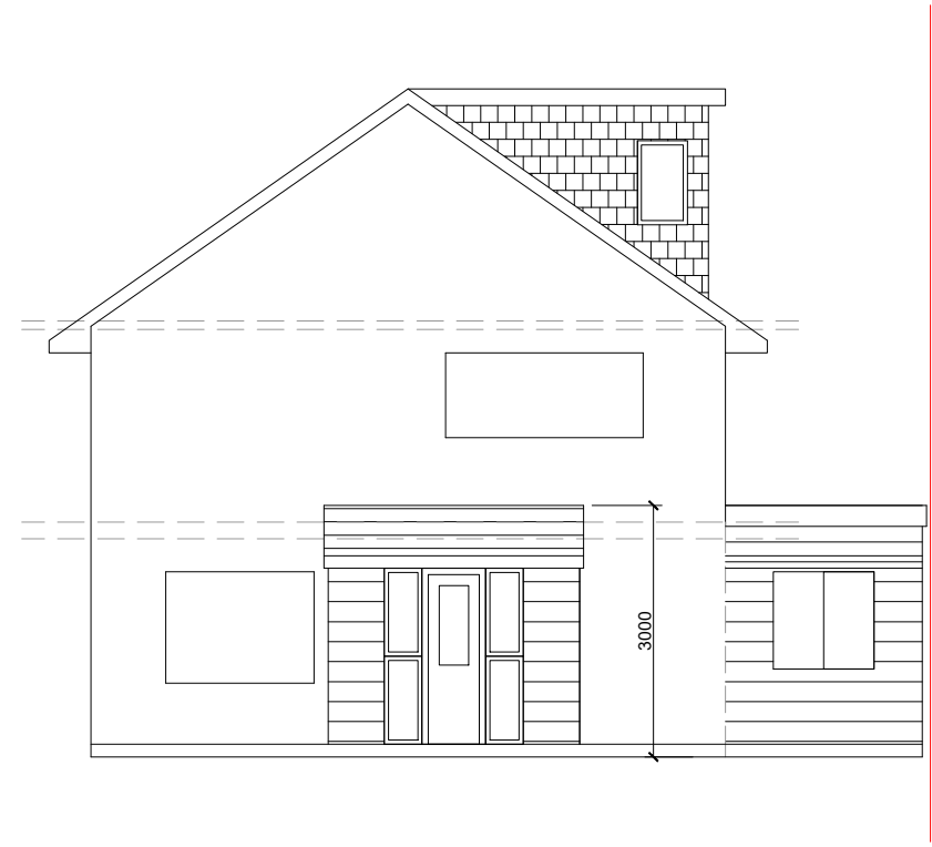
PROPOSED FRONT ELEVATION Scale 1:100
