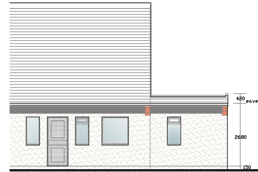
SIDE ELEVATION A AS PROPOSED 1:100
