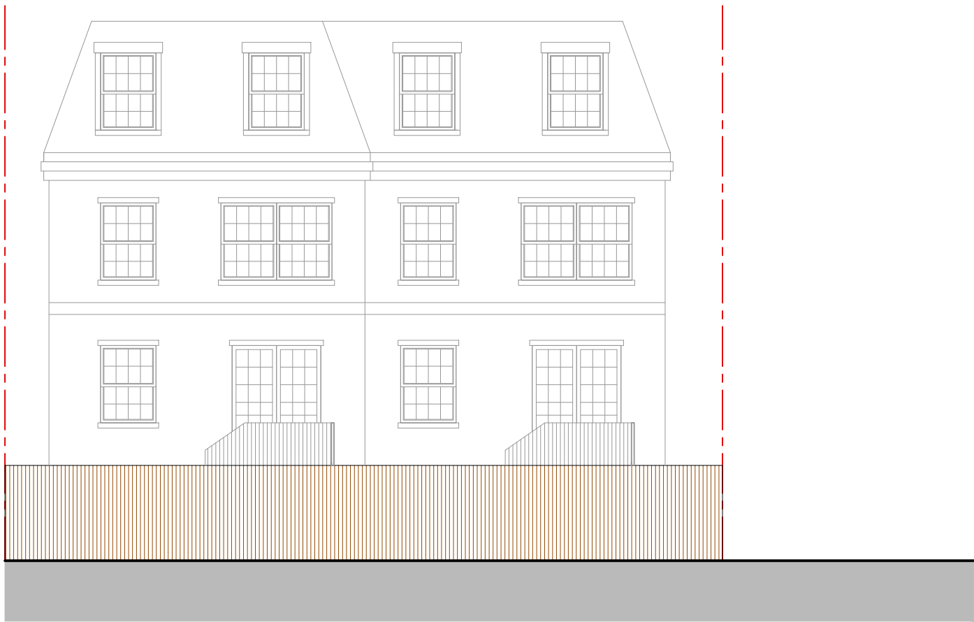
Proposed Rear Elevation Scale 1:100
