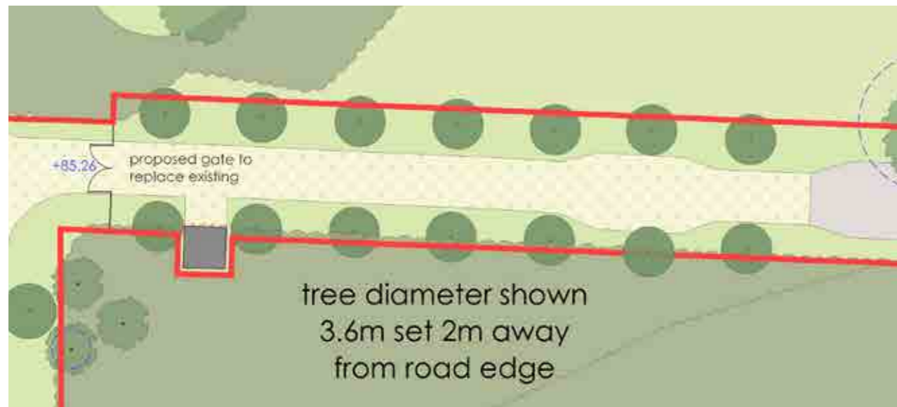
Section of landscape plan showing entrance avenue area. A zone for a proposed substation is shown to the left hand side to the entrance gate and screened to the avenue approach by proposed trees.
