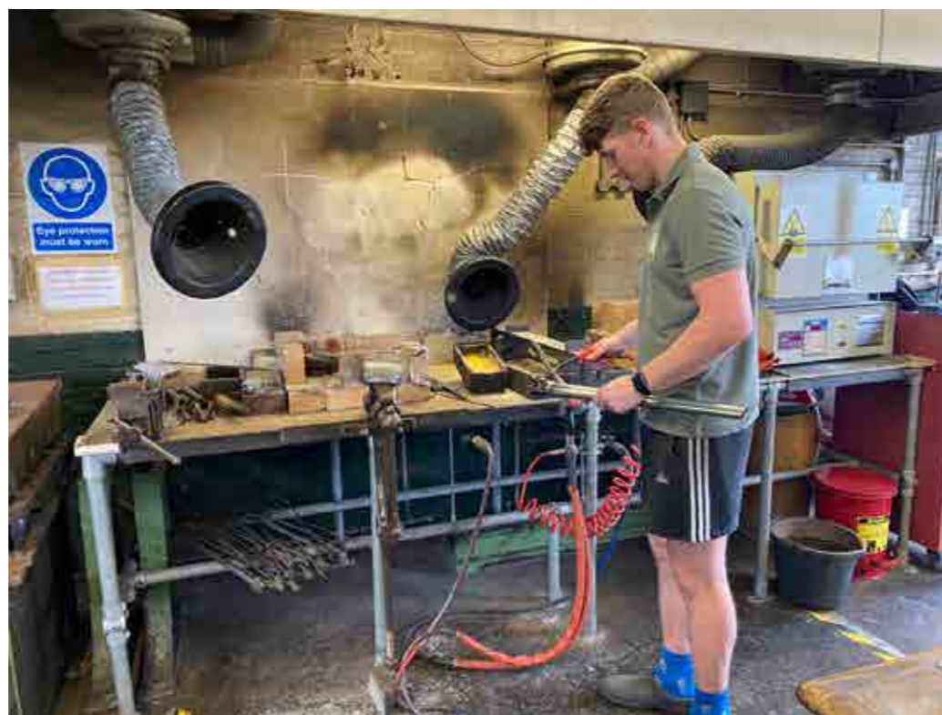
Hot-works area being used for gun barrel fabrication
