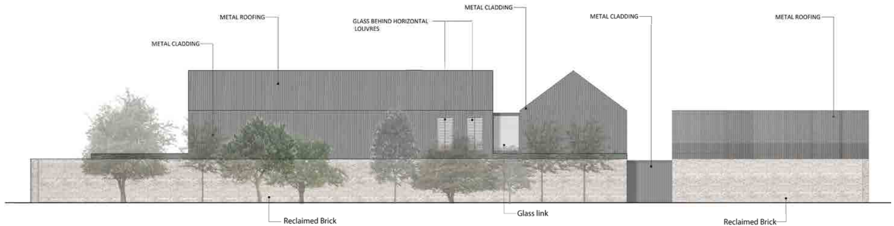
Illustrated South Elevation : Reclaimed brick 'garden wall' at low level and metal cladding above. The facade concept is based around a consistent masonry datum with metal cladding above to provide both articulation and unity to the overall assemblage. A host of proposed trees will provide additional screening to the South boundary as can be seen in the illustration.
