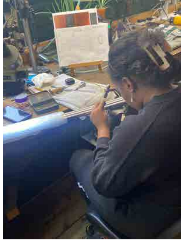
Gun barrels being engraved by hand
