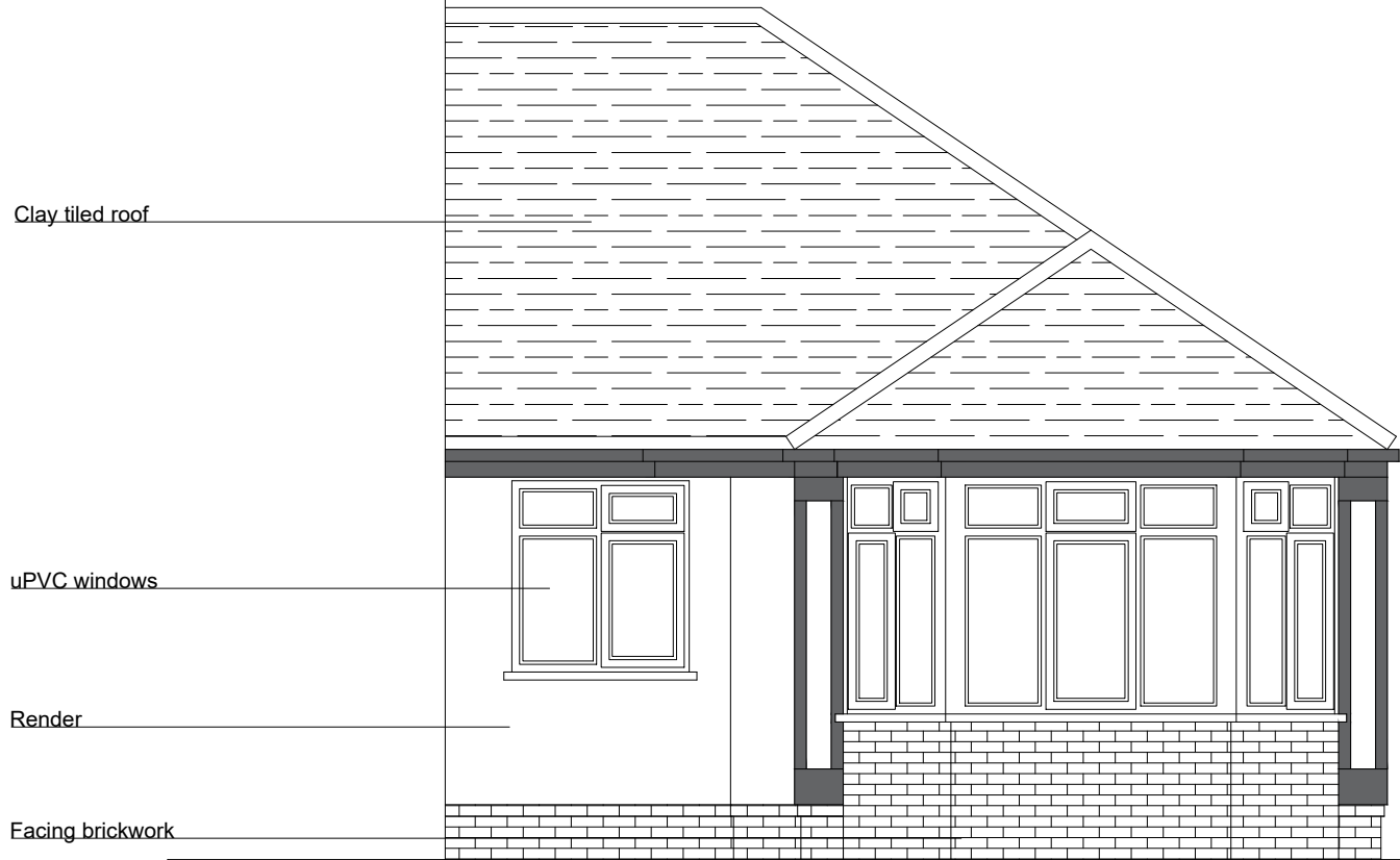
EXISTING FRONT ELEVATION C
