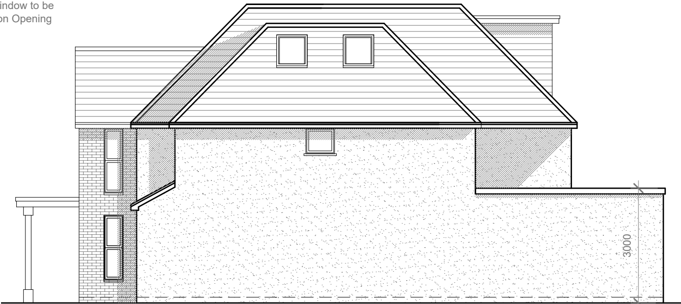
Proposed Side Elevation Scale 1:100
