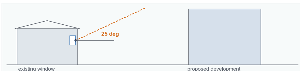
The 25-degree screening test: where any part of the proposal rises above a line drawn at 25 degrees from the centre of the lowest neighbouring window, the detailed VSC tests are undertaken.
