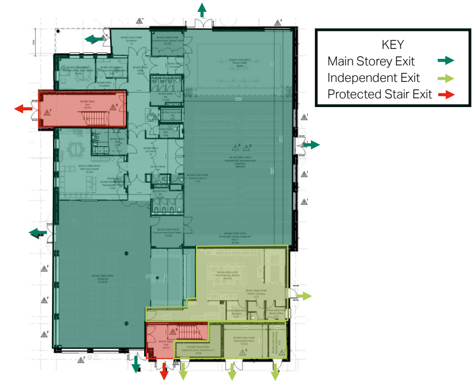
Figure 4: Ground Floor Storey Exits
