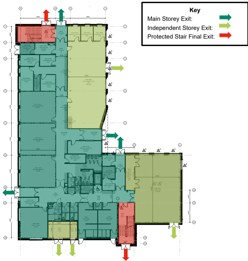
Figure 3: Ground Floor Final Exits
