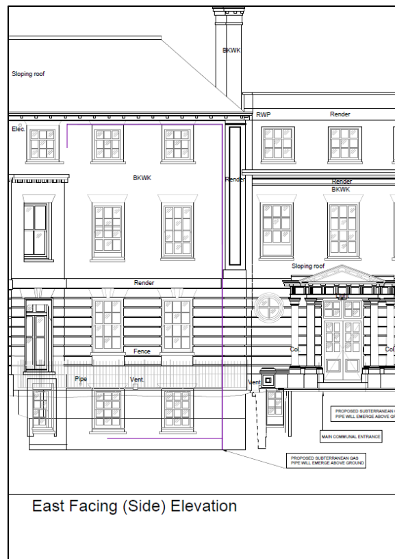
Plate 4: Indicative route of pipework on (east facing elevation of Cowley House
