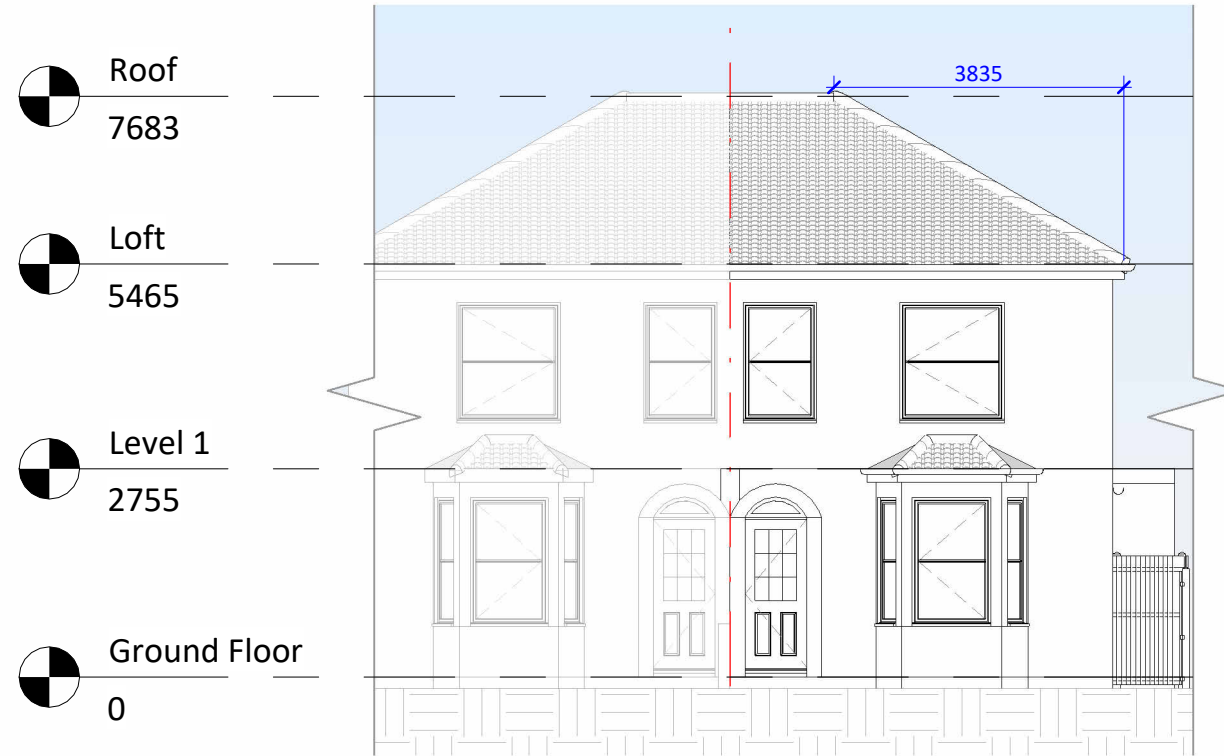
1 Existing Front Elevation 1 : 100
