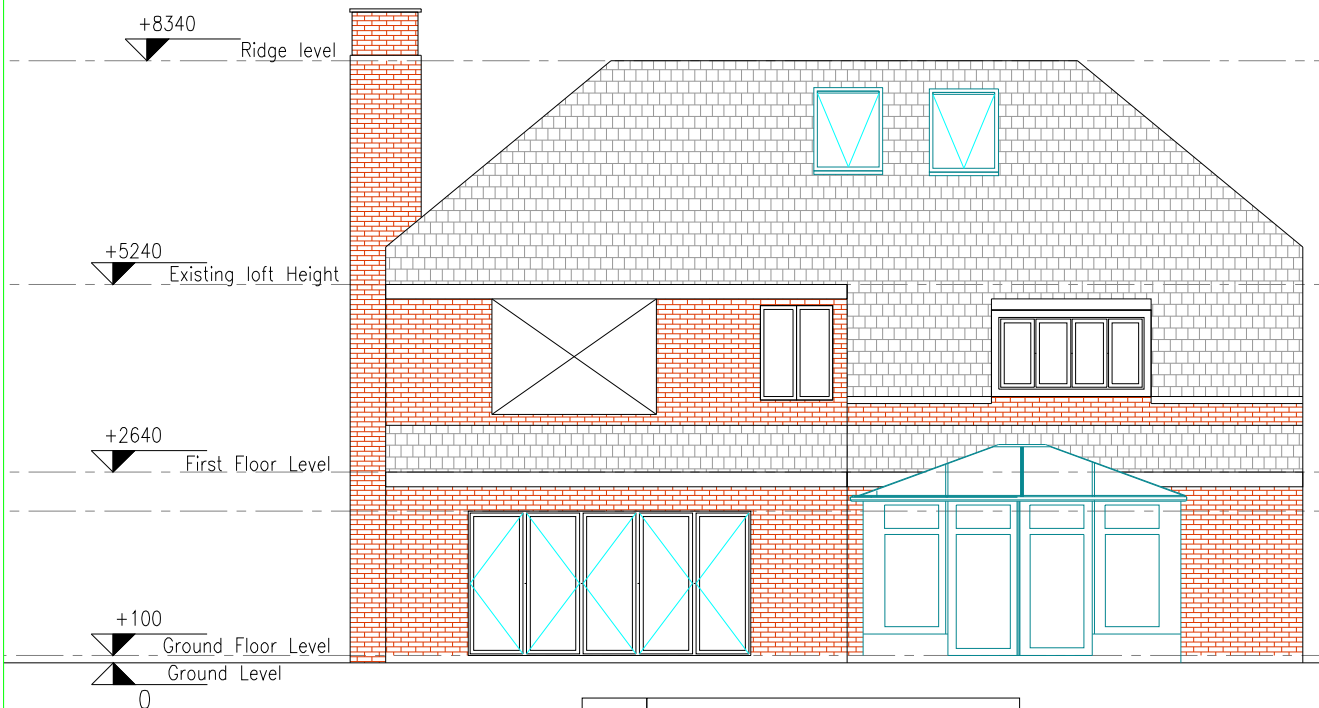
12 EXISTING REAR ELEVATION
