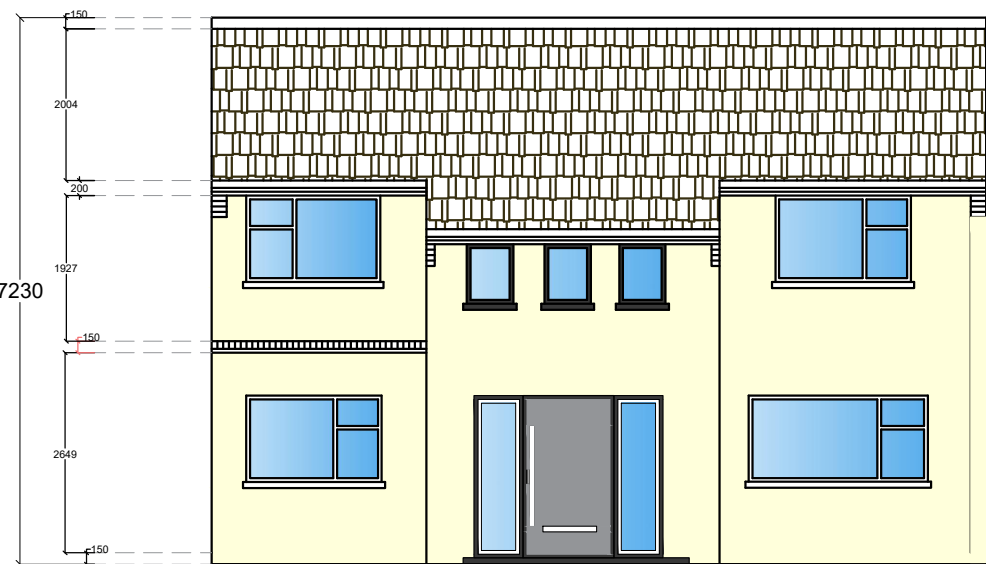
PROPOSED FRONT ELEVATION SCALE 1:100
