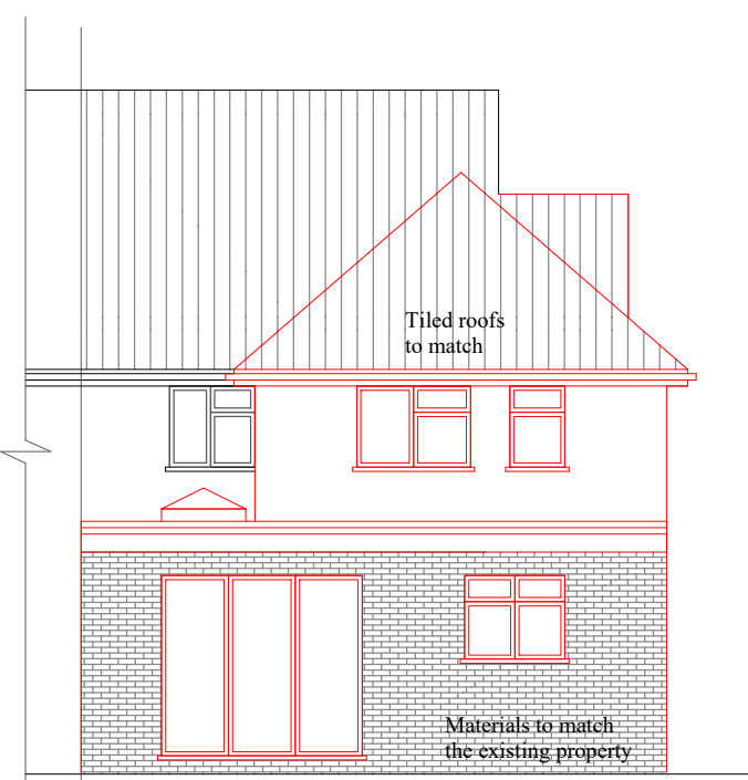
PROPOSED REAR ELEVATION
