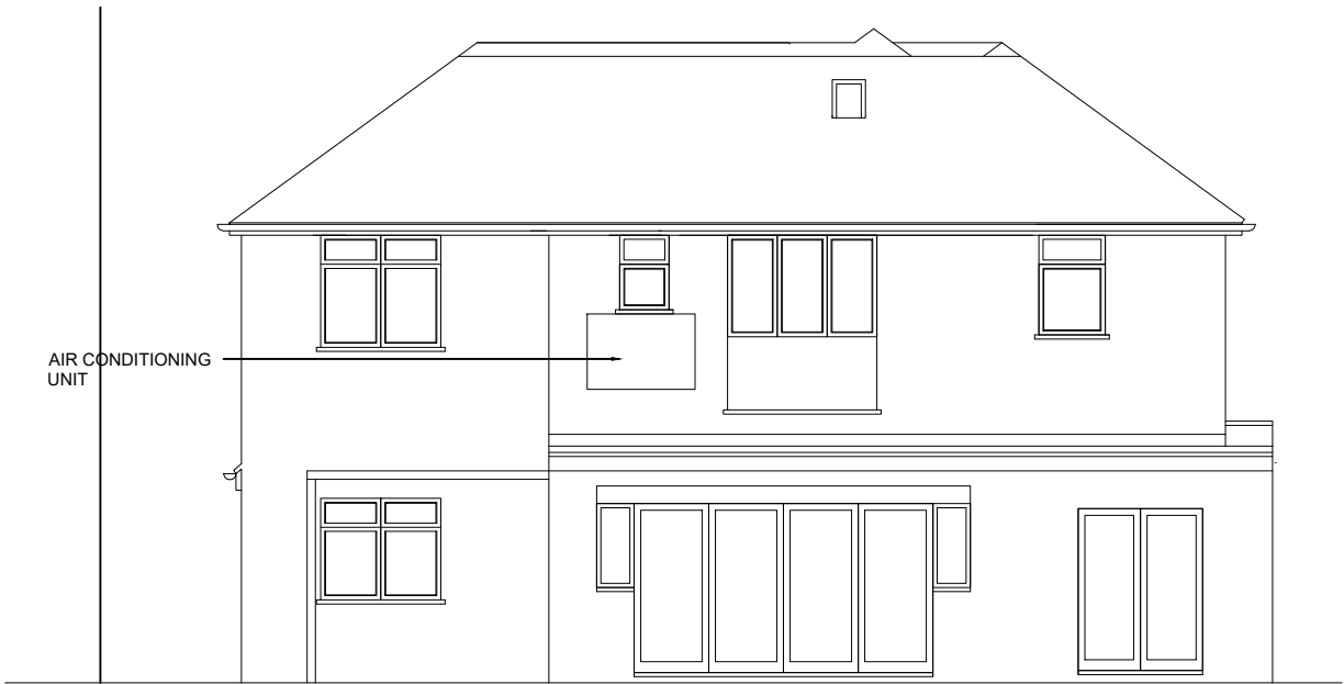
As Built Rear Elevation
