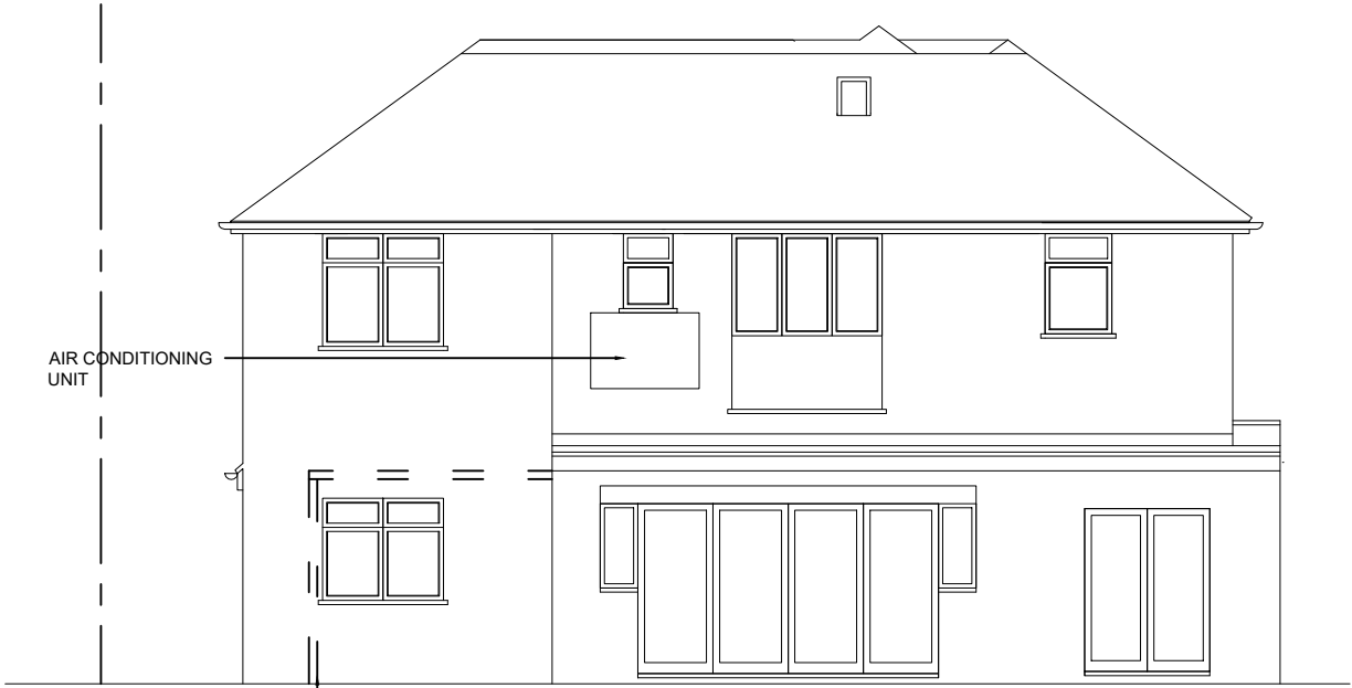
As Built Rear Elevation
