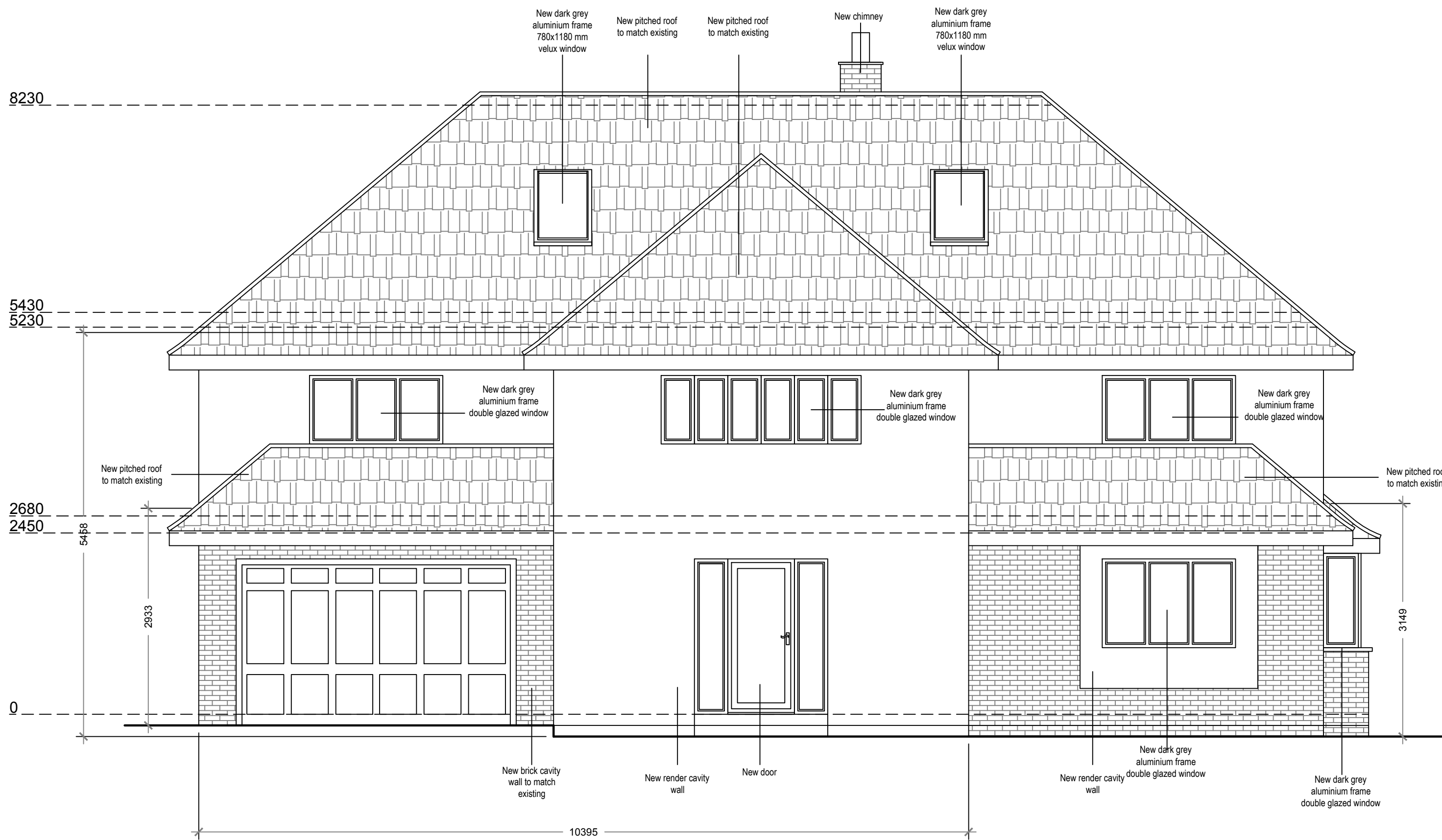
Proposed Northeast Elevation Scale 1:50
