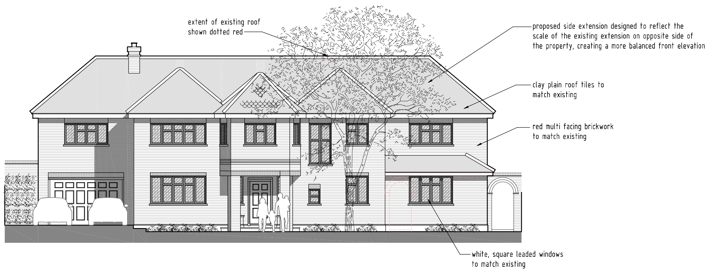
PROPOSED FRONT ELEVATION SCALE 1:100
