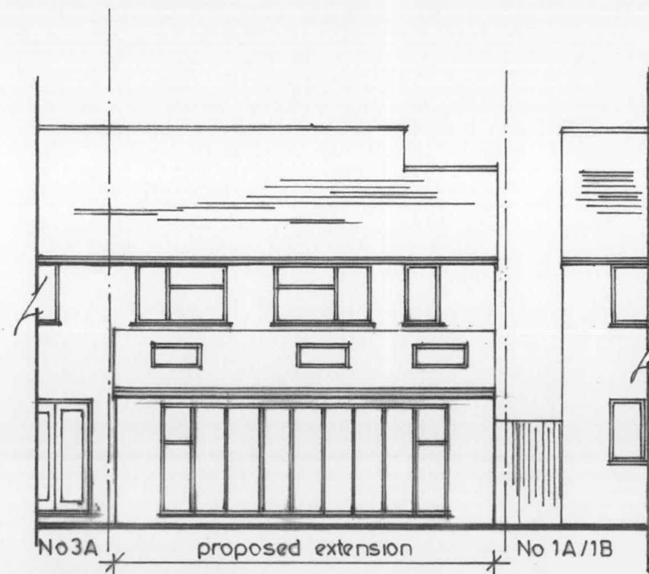
REAR ELEVATION External materials to match existing
