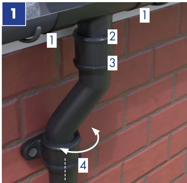
Where square or rectangular pipes are being installed and offsets are required, alignment between the gutter outlet and gully must be exact. Round pipe systems are more flexible to install and offsets can be adjusted and 'swung' into alignment with the gully position.
