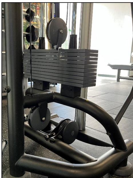
Photo 4: Rubber stops on weight stacks
