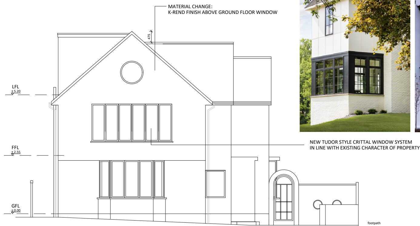
1 | PROPOSED LEFT SIDE ELEVATION SCALE 1:100
