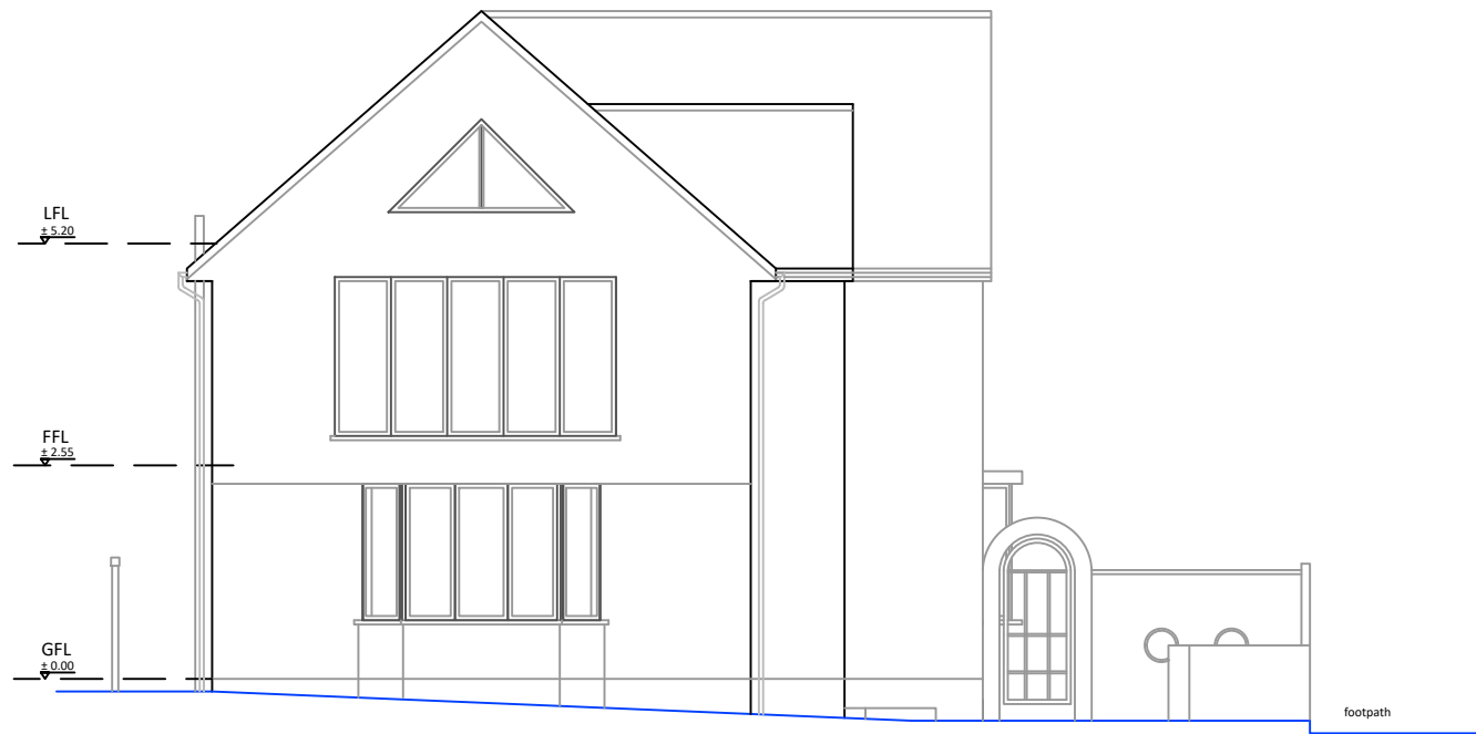
1 | PROPOSED LEFT SIDE ELEVATION SCALE 1:100
