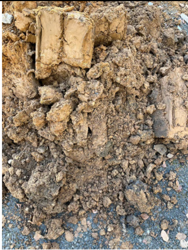
TP203 arisings (Langley Silt Member)
