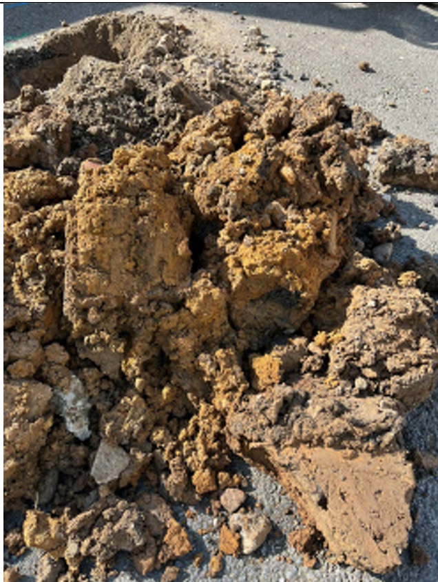
TP202 arisings (Langley Silt Member)
