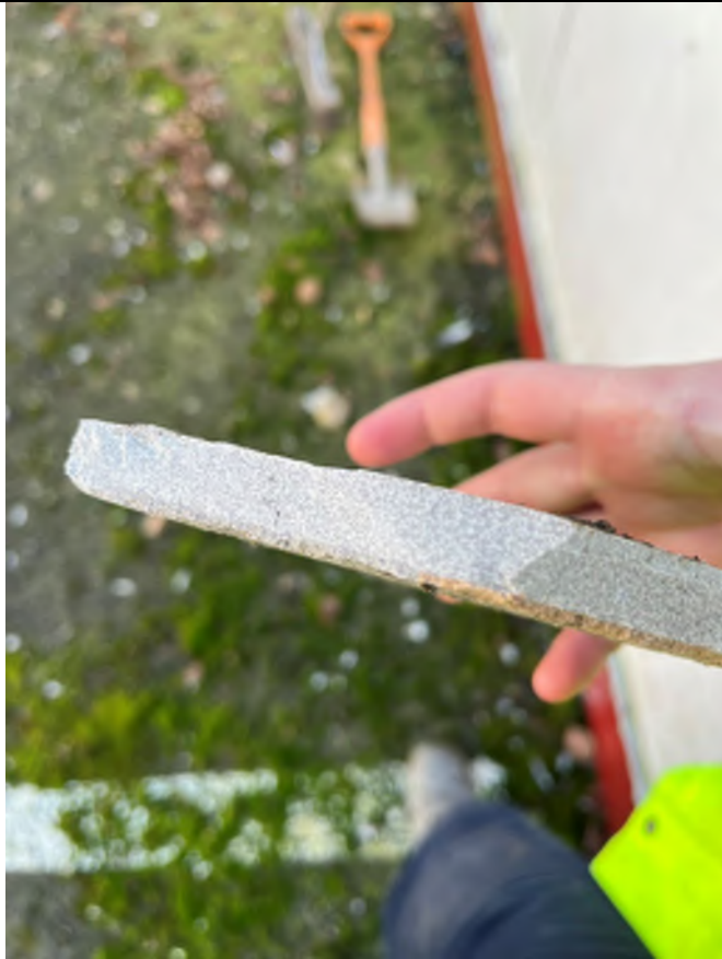
TP203 tiling found immediately below hardstanding
