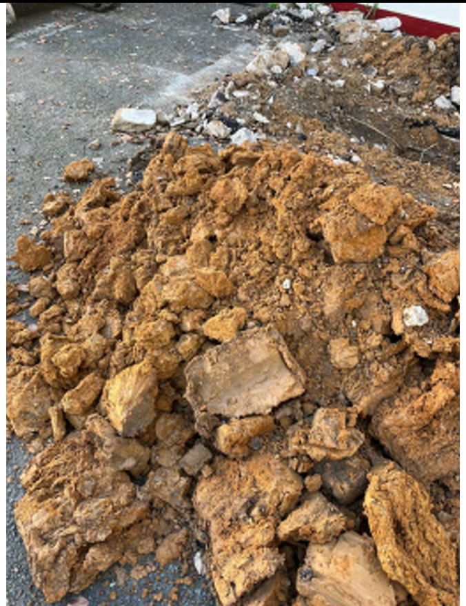
TP203 arisings (Langley Silt Member)
