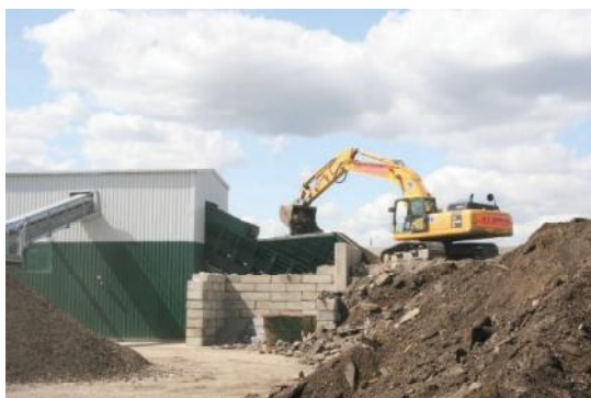
Arising fed into our static crusher housed in an acoustic silenced building
