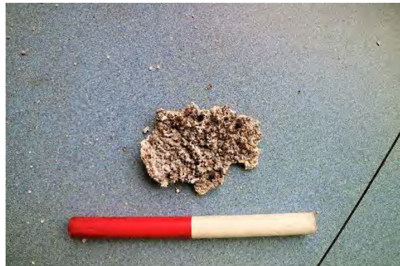
Fig 39 Detail shots of the sound proof cement render ceiling
