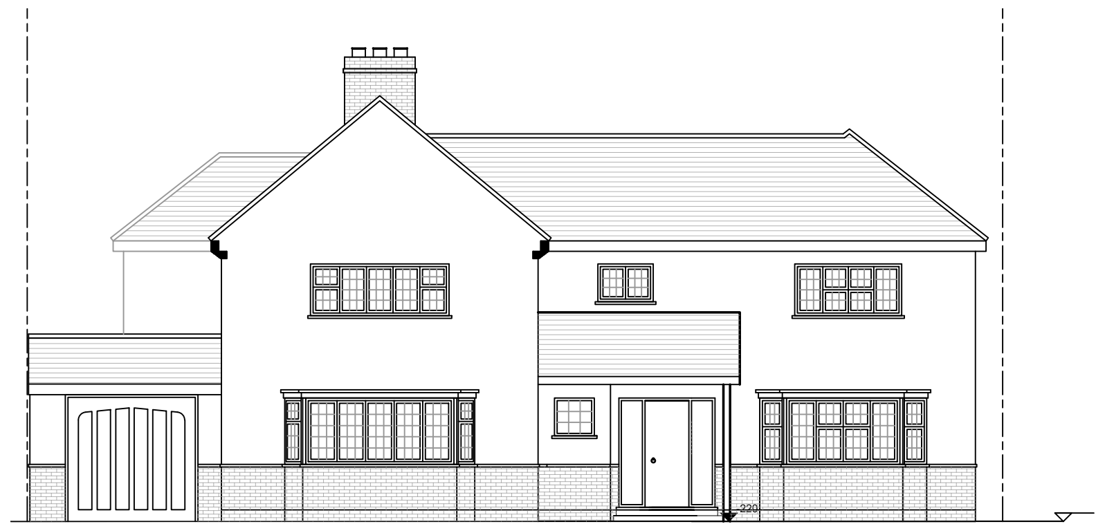
PROPOSED FRONT ELEVATION SCALE 1:100
