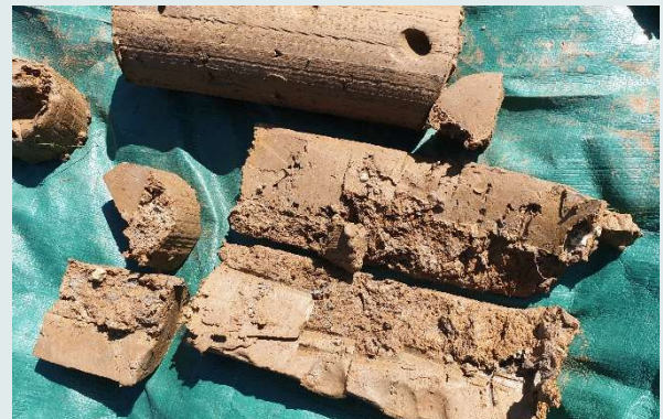
Core of London Clay from WS07
