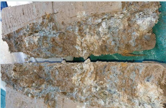
Core of London Clay from WS04
