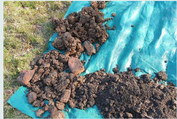
Made Ground from WS12 with brick cobbles
