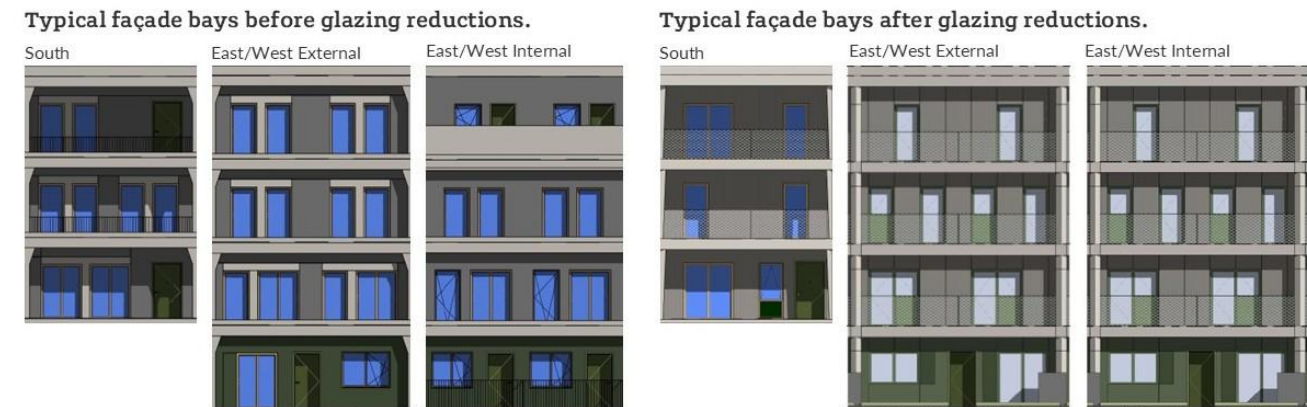
Figure 5: During the RIBA Stage 2 design process, the glazing ratios have been significantly reduced to minimise overheating (Credit: SEW Architects)..Suitable g-values have been specified to further control solar heat gains as required.
