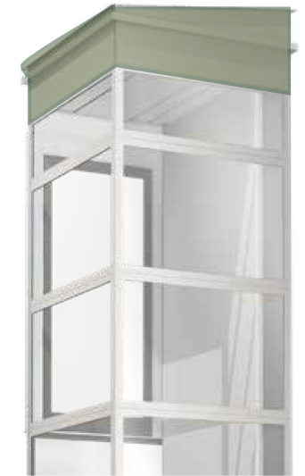
Proposed glass envelope to external lift to provide additional safety and security. Modular system allowing for site adjustment as necessary.
