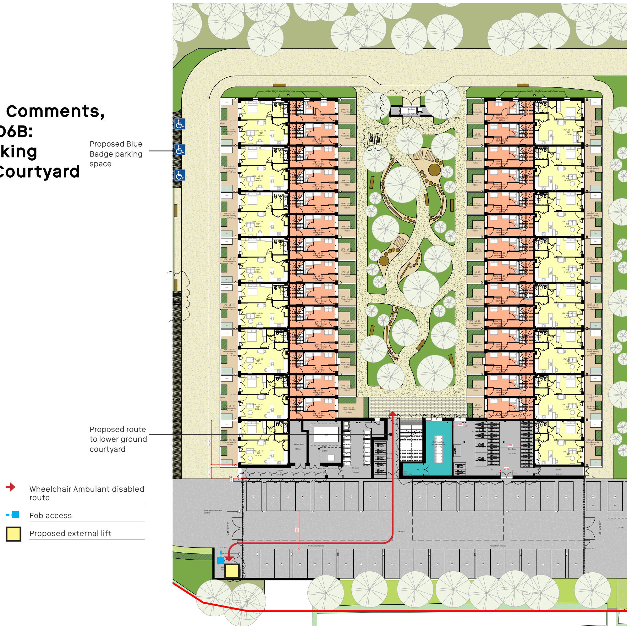
Proposed Lower ground floor plan showing wheelchair / ambulant disabled user access to the external platform lift and the courtyard
