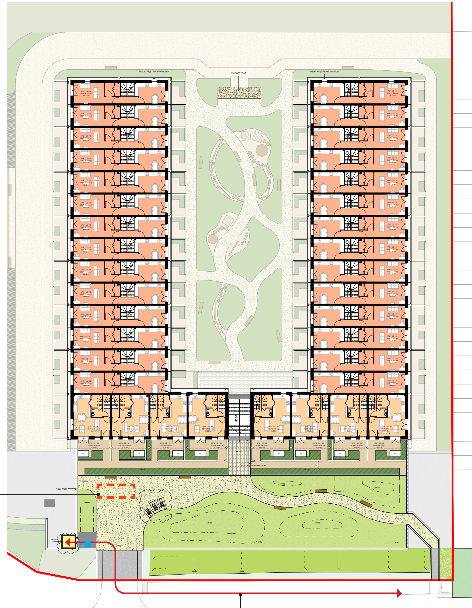
Proposed Ground floor plan showing wheelchair / ambulant disabled user access to the external platform lift
