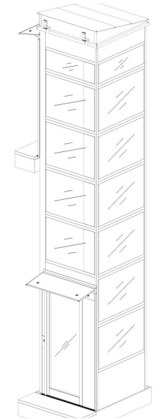
Proposed glass envelope to external lift to provide additional safety and security. Modular system allowing for site adjustment as necessary.
