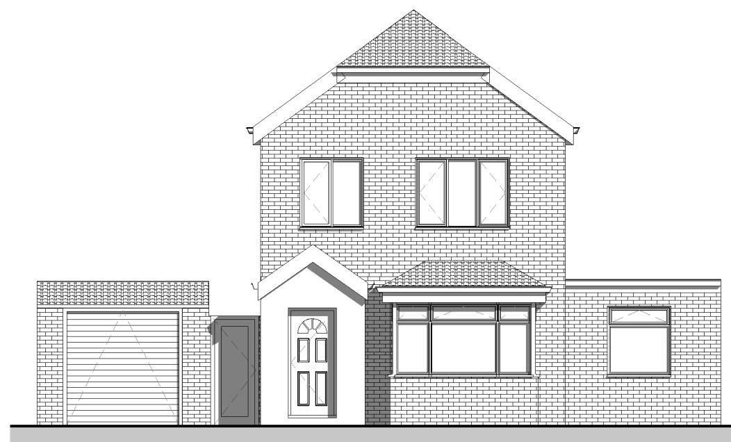
3 Existing Front Elevation 2112-A-500 1 : 100
