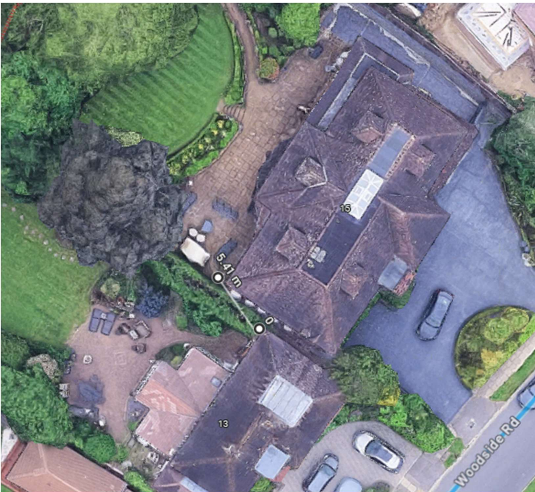
Figure 3. Distance between the proposed basement corner and the corner of the existing neighbours building
